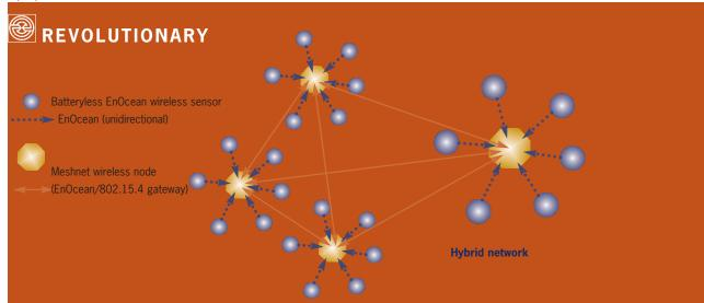
EnOcean technology is the ideal addition to wireless networks to create batteryless and maintenance-free, wireless sensor networks
