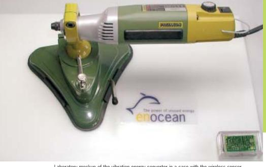
Laboratory mockup of the vibration energy converter in a case with the wireless sensor.
