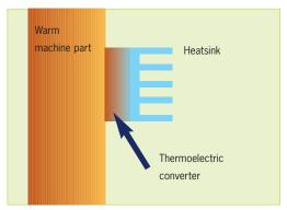
Schematic of thermal energy converter
