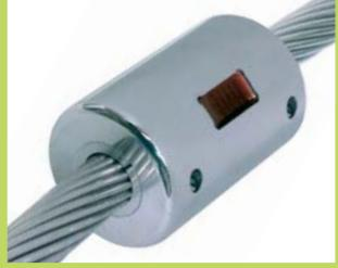
Study for a solar-powered wire monitoring sensor
