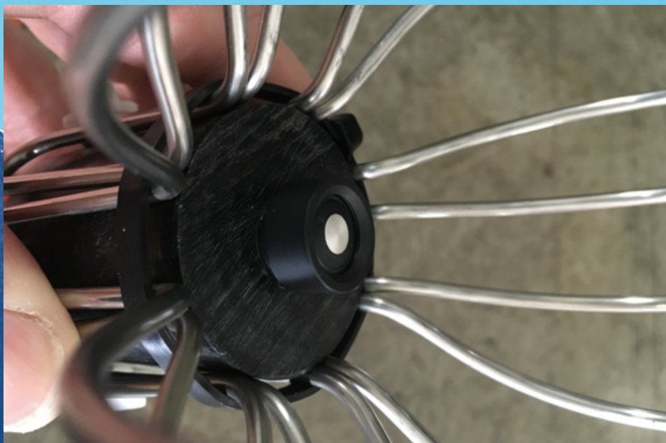
The Echoponics DOS (Dissolved Oxygen Sensor) from Echoflex Solutions uses the EnOcean signal to wirelessly transmit data about water characteristics.
