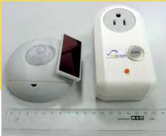
Demonstrator: power outlet receiver with turn-on button.
