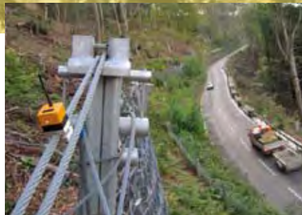
Impact Sentinel is a wireless supported system used by Swiss Federal Railways to observe rockfall.
