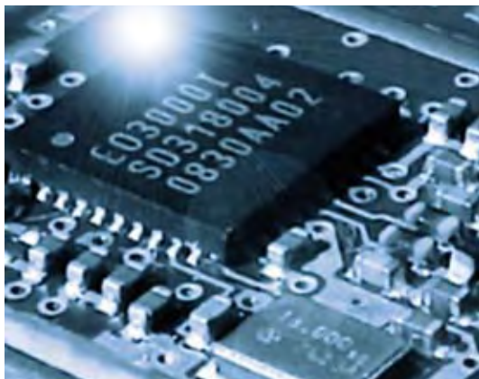
EnOcean Dolphin ASIC EO3000I on a board
