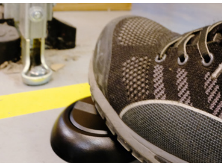
Employee using the Floor Switch to open motorized gates.
